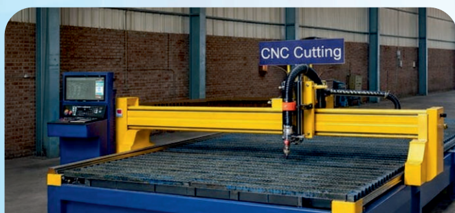
CNC Plasma Cutting Machine Up to 30 mm with Plasma & 150 mm with Oxyfuel
